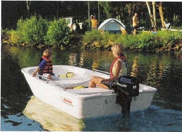
Figure 1-21. The qualities valued most in a utility outboard are stability and load-carrying ability, achieved in this boat in part with a blunt, skiff-like bow. (COURTESY BOSTON WHALER)
