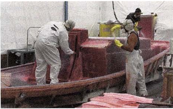
Figure 1-35. A fiberglass boat under construction. (COURTESY NATIONAL MARINE MANUFACTURERS ASSOCIATION)
