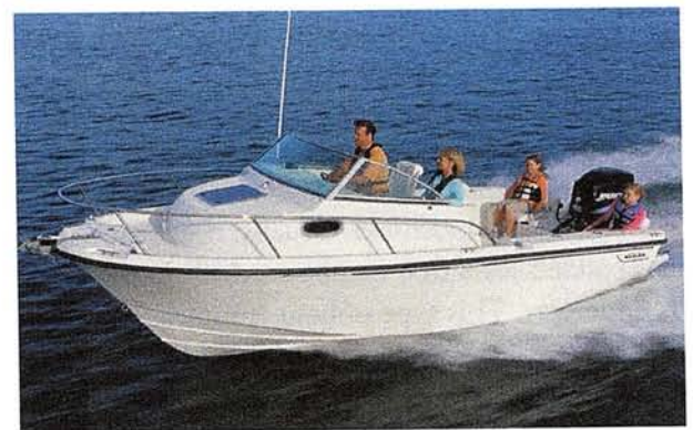
Figure 1-26. A cuddy cabin offers shelter and creature comforts but impedes access to the foredeck. (COURTESY BOSTON WHALER)
