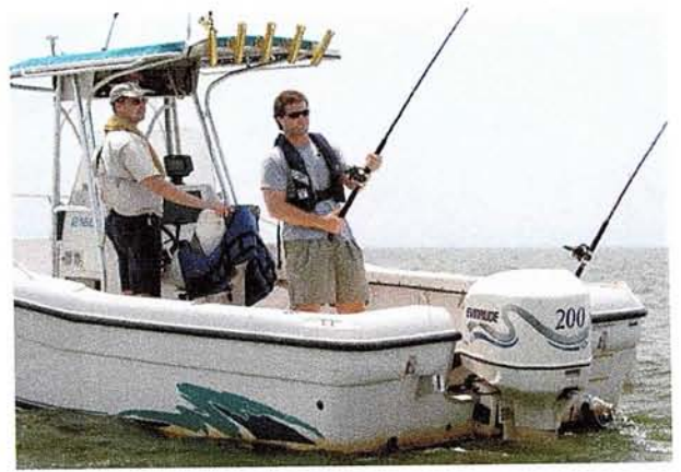
Figure 1-25. A center console fishing boat—the cockpit provides protection from the sun. Rod holders on the hardtop are another feature shown here. (COURTESY COAST GUARD AUXILIARY)
