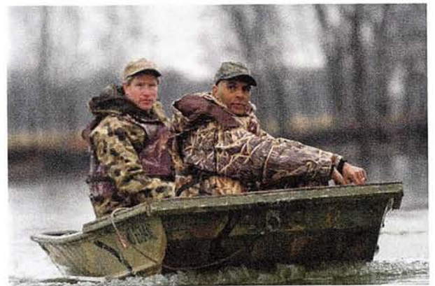
Figure 1-20. An aluminum jonboat with camouflage paint for duck hunting. (COURTESY U.S. COAST GUARD OFFICE OF BOATING SAFETY)
