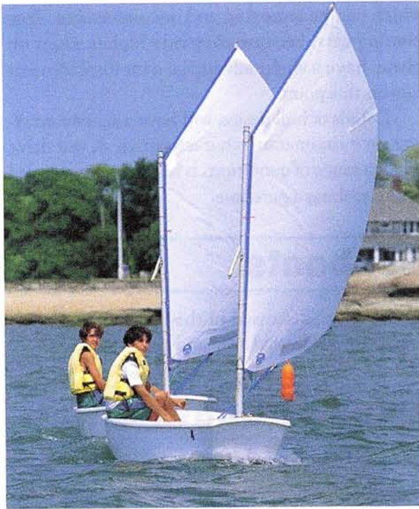
Figure 1-18. Two sailing prams underway. The Optimist class of prams, which are very much like these, are raced worldwide. Prams without sailing rigs, built for rowing, serve as stable, inexpensive tenders for larger boats. (COURTESY NATIONAL MARINE MANUFACTURERS ASSOCIATION)
