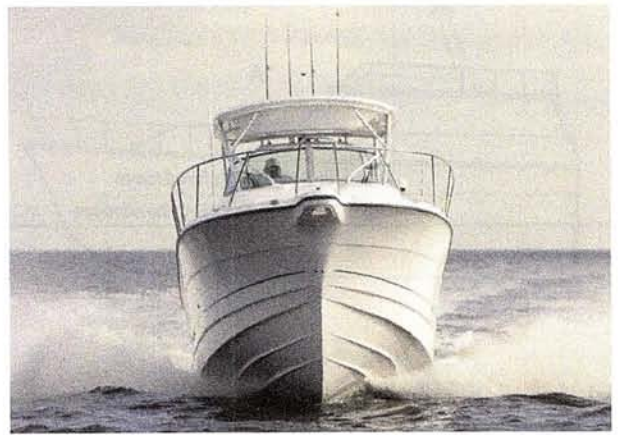
Figure 1-14. This approaching powerboat shows two running strakes beneath a chine flat on either side. These features add lift for planing as well as side-to-side stability. (COURTESY BAYLINER)
