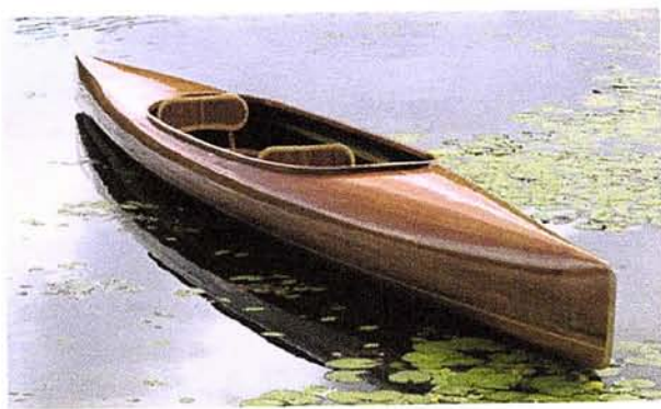
Figure 1-34. A strip-built tandem canoe, suitable for home construction. (COURTESY NICK SCHADE)
