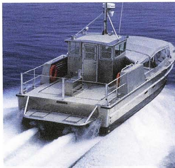
Figures 1-13. Top and middle: Two planing powerboats skimming over the water in ideal conditions. (COURTESY U.S. COAST GUARD OFFICE OF BOATING SAFETY) Bottom: A commercial vessel with twin jet drives on plane. (COURTESY HAMILTON JET)
