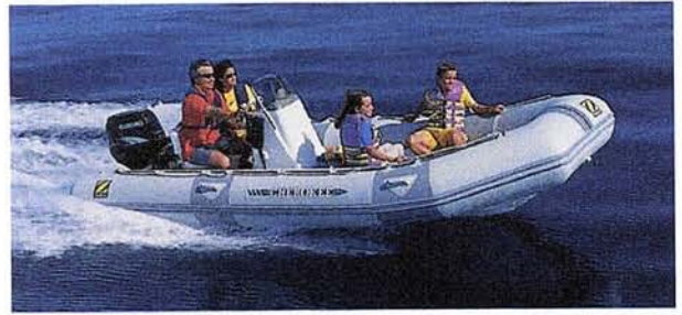
Figure 1-19. A rigid inflatable boat (RIB) provides excellent buoyancy and stability with lower weight than a conventional fiberglass boat of similar size and capacity. (COURTESY ZODIAC)
