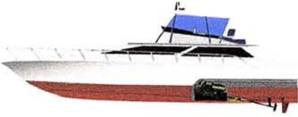
Figure 1-8. Cutaway view of an inboard engine installation. This boat has twin engines, each with its own driveshaft and propeller, and twin rudders. (REPRINTED WITH PERMISSION FROM AMERICA'S BOATING COURSE, PUBLISHED BY BOAT ED)
