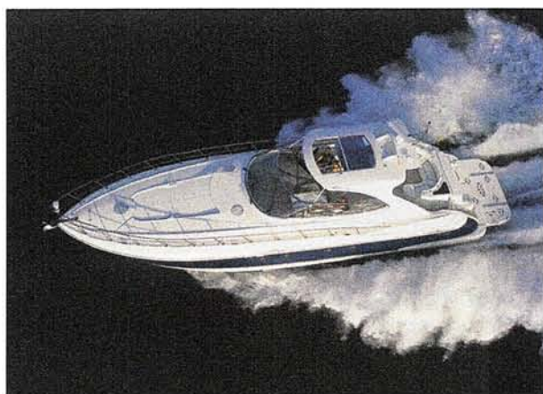
Figure 1-16. A semidisplacement hull at speed, showing separation of the wake around the transom. (COURTESY CRUISERS YACHTS)
