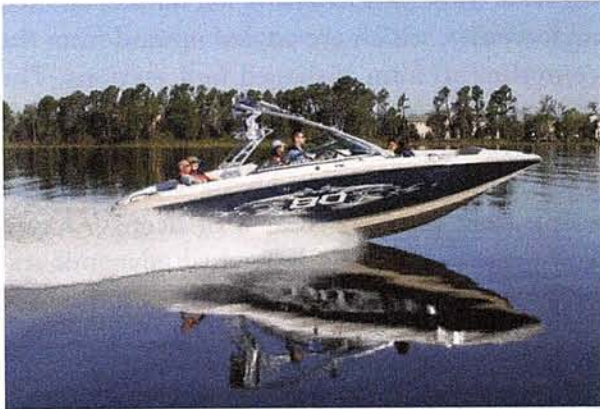
Figure 1-14. This approaching powerboat shows two running strakes beneath a chine flat on either side. These features add lift for planing as well as side-to-side stability. (COURTESY BAYLINER)
