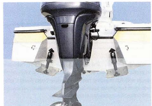
Figure 1-15. A stern-view illustration showing trim tabs slightly lowered to help a powerboat get on plane. For more on trim tabs, see Chapter 4. (COURTESY LENCO MARINE)
