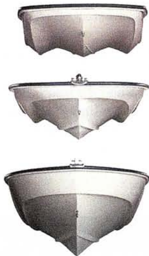
Figure 1-24. In the Boston Whaler line of boats, the smaller models—13 feet and under—derive much of their stability from the sponsons of a cathedral hull form (top). The 15- to 17-foot models (middle) derive more stability from their greater hull width, so the sponsons can be reduced in favor of a deeper-V central hull that offers smoother rough-water performance. This trend continues in the 18-foot and longer boats (bottom), with the sponsons replaced by chine flats. (COURTESY BOSTON WHALER)
