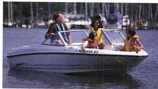
Figure 1-23. A bowrider, showing the walkthrough windshield that is characteristic of the type. (COURTESY BAYLINER)
