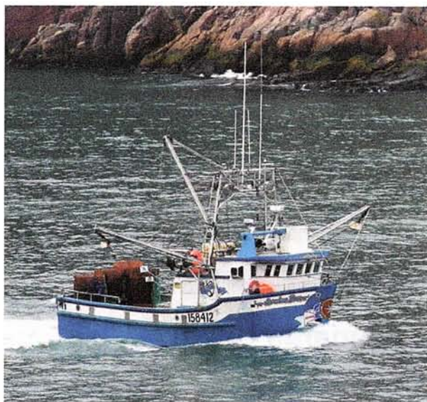
Figure 1-12. Left: This fishing vessel in St. John's, Newfoundland, shows how much water a displacement powerboat pushes aside at cruising speed. Any further incremental speed increase is gained only at the cost of greatly increased fuel consumption. Right: A sailboat is also a displacement hull. (LEFT PHOTO BY JIM BARTLETT, COURTESY NATIONAL MARINE MANUFACTURERS ASSOCIATION. RIGHT PHOTO COURTESY SPECTRUM PHOTO/FRAN GREON)
