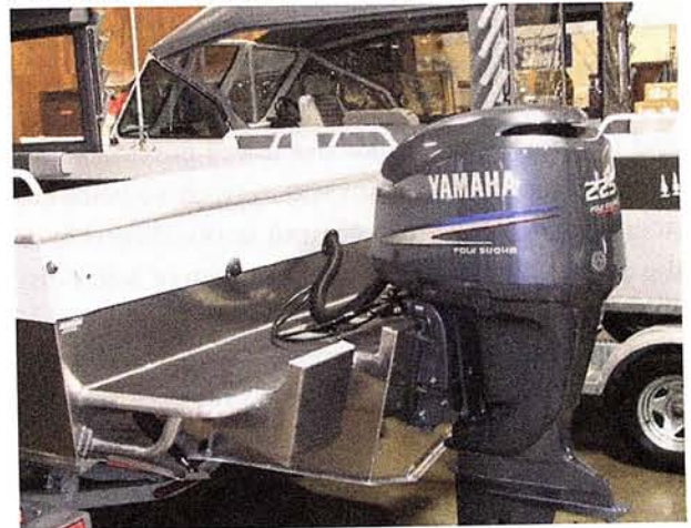
Figure 1-7. Mounting an outboard engine on a bracket aft of the transom permits a full transom and unimpeded interior volume. (PHOTO BY ED SWEENEY)
