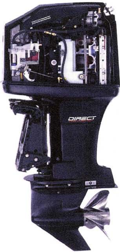
Figure 1-5. This cutaway view of a direct fuel-injected 200-horsepower outboard hints at the complexity of a modern outboard motor. (COURTESY MERCURY MARINE)
