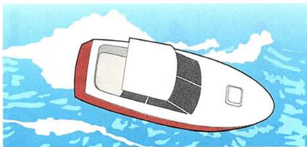
Figure 4-55. On the other hand, taking the seas on the beam will subject your boat to uncomfortable rolling, and may even put it at risk of capsizing if the seas are steep and high enough.
