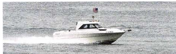
Figure 4-35. Top to bottom: A powerboat traveling at slow speed, getting up on plane (note squatting stern and bigger wake), and planing (level keel, smaller wake). (PHOTOS BY BOB DENNIS)
