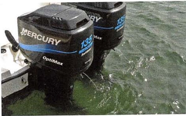
Figure 4-20. The telltale cooling water streams coming from these idling outboard motors show that the cooling water flow is normal. (PHOTO BY BOB DENNIS)
