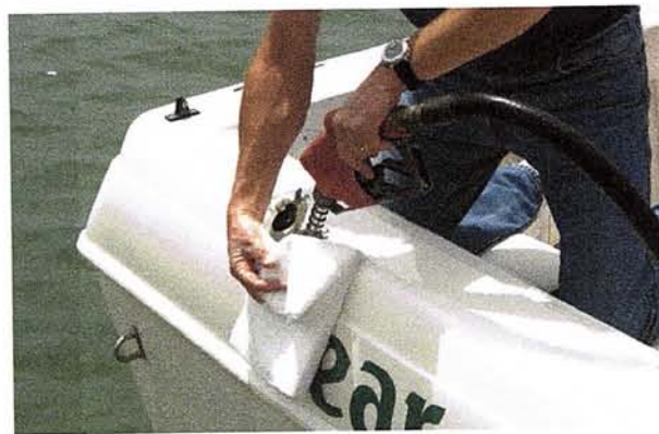
Figure 4-1. Refueling at the marine dock. Note the use of an absorbent pad to prevent spills. (PHOTO BY BOB DENNIS)
