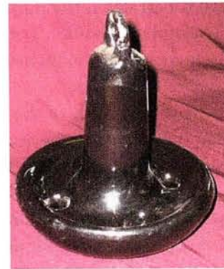
Figure 4-47. Small mushroom anchors like this one are sometimes used by anglers, but larger mushrooms are used mainly for permanent moorings, as they must sink into the sediment before they are effective.
