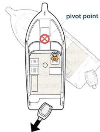
Figure 4-10. A turning boat pivots about a point a third of the way back from the bow.
