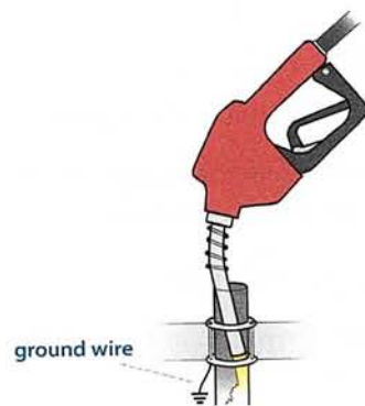
Figure 4-2. When refueling, keep the nozzle in contact with the filler pipe to prevent static electricity buildup.
