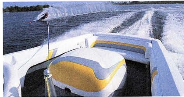
Figure 4-52. This water-skier’s tow rope is fastened to a towing pylon on the boat. (COURTESY NATIONAL MARINE MANUFACTURERS ASSOCIATION)
