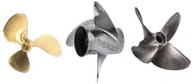
Figure 4-6. Left to right: A three-bladed propeller for an inboard engine. (COURTESY MICHIGAN WHEEL) A three-bladed stern-drive or outboard propeller. (COURTESY JOHNSON) A four-bladed prop can deliver less vibration and more blade area in a given diameter than a two- or three-bladed propeller, though with some loss of efficiency. (COURTESY BOMBARDIER RECREATIONAL PRODUCTS)
